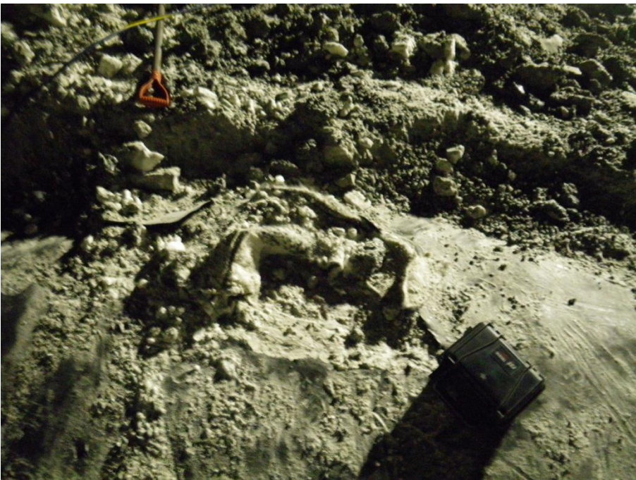
Photo 11: Tear in GCL observed at station 1+55 note the RST readout box for scale.
